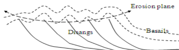
Fig.2: Schematic diagram for repetition of Disangs in imbricate slices with folding of upper layers on top
